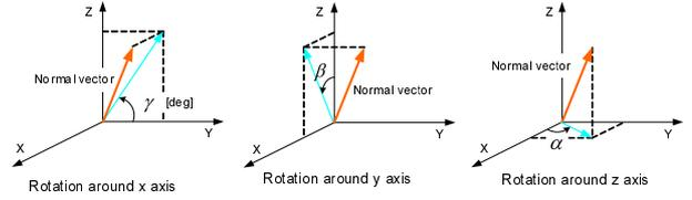
Fig. 10. Roll-pitch-yaw angle
