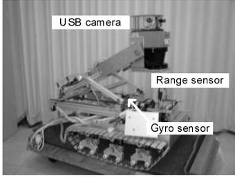
Fig. 2. Target robot (Res-Dog)
