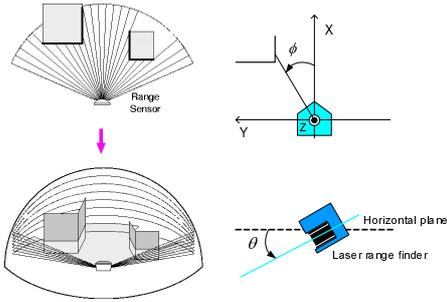
Fig. 3. Acquisition of three-dimensional environment data
