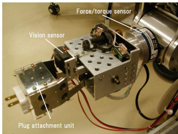
Fig. 6. Plug attachment unit and force/torque sensor
