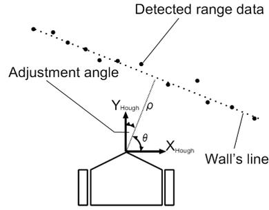
**Fig. 9.** Adjustment motion using Hough transform method
