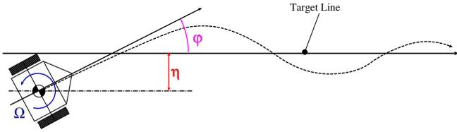
Fig. 5. Image of the control law to make wheeled-type vehicles follow the given target straight line
