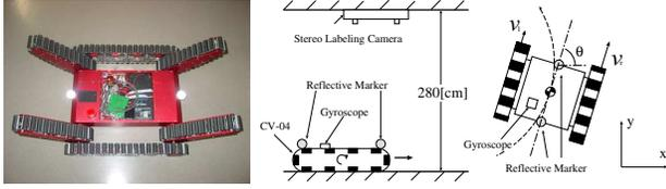
Fig. 2. Tracked vehicle and experimental setup
