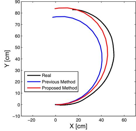
Fig. 4. Real and estimated trajectories of the vehicle following a curve using a p-tyle(at  $v_r = 15.0$ [cm/sec],  $v_l = 1.9$ [cm/sec])
