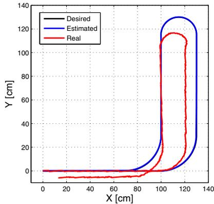
Fig. 9. Results based on “odometry with a gyro”
