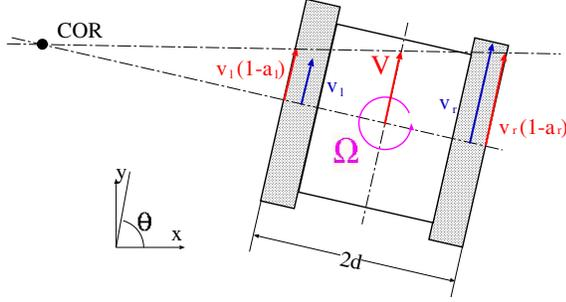
Fig. 1. Kinematic model for tracked vehicles
