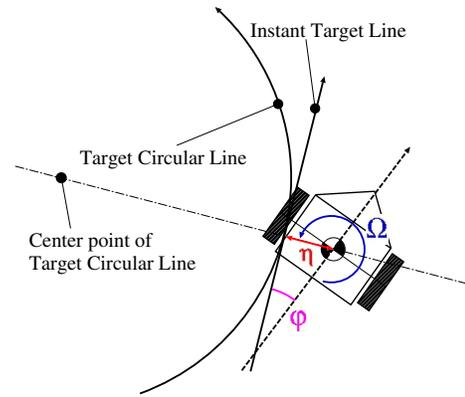
Fig. 6. Image of the control law to make wheeled-type vehicles follow the given target circular line
