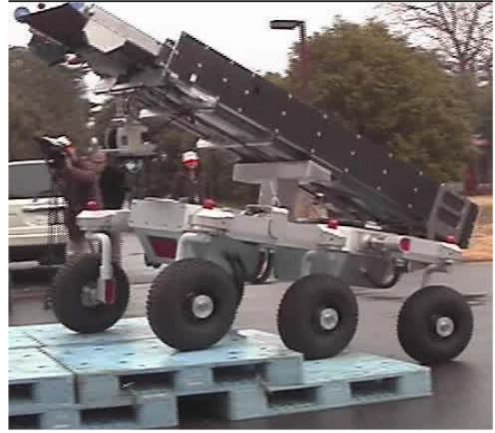
Fig. 6. A performance test of surmounting steps for large robot
