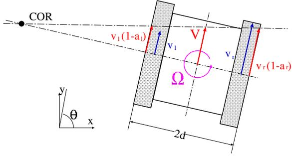
Fig. 2. Kinematic model for tracked vehicles
