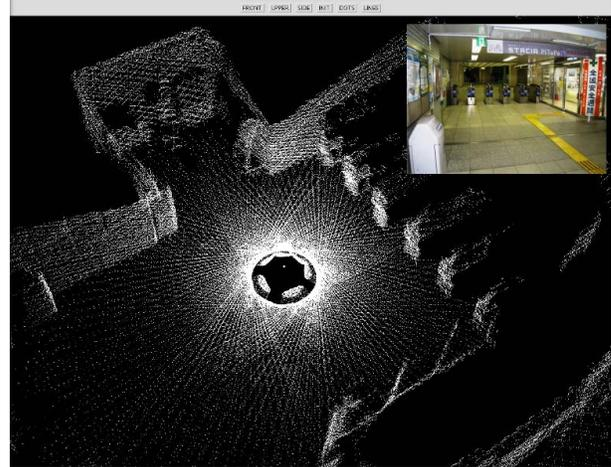
Fig. 9. Scan result with robot's rotational motion
