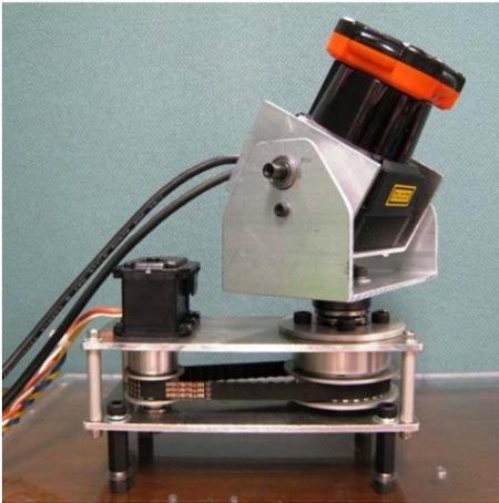
Fig. 6. three-dimensional laser range scanner
