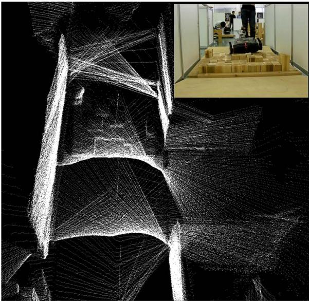
Fig. 10. Scan result with robot's traversing motion on step field
