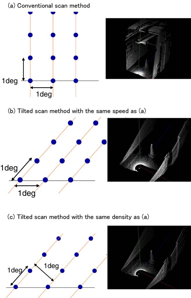
Fig. 7. Comparison of scan-speed and scan-density
