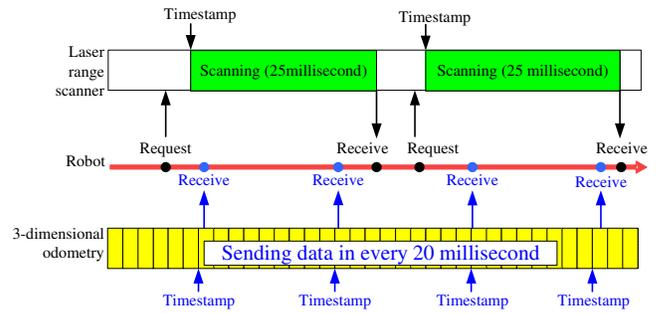
Fig. 8. Synchronization between scanning data and odometry
