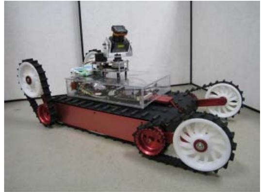
Fig. 1. Tracked vehicle testbed Kenaf-II
