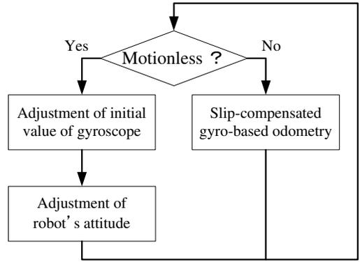
Fig. 3. A concept of compensation of gyroscope's drift
