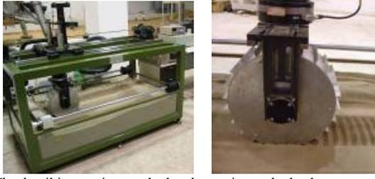
Fig.6 Wheel-soil interaction test bed and experimental wheel. Different metal wheels with different radii, widths and lugs were used, as shown in Table I, where  $n_L$  is the number of wheel lugs.
