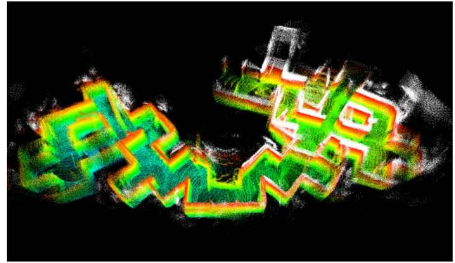
(a) Odometry mapping (3D mapping based on odometry)
