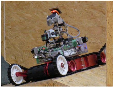
Fig. 2. Tracked vehicle Kenaf 22 with 3D range scanner (at the top)
