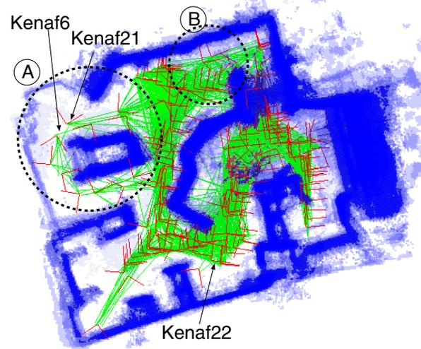
(c) Corrected map using data obtained by all three robots
