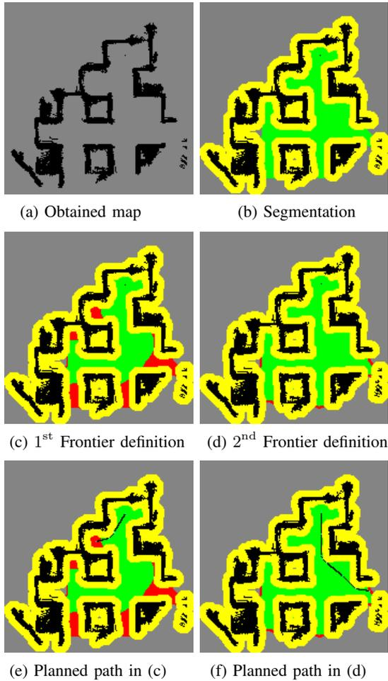
Fig. 5. Frontier-based coverage path planning
