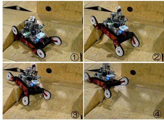
Fig. 3. Maintaining stability by autonomous control of sub-tracks
