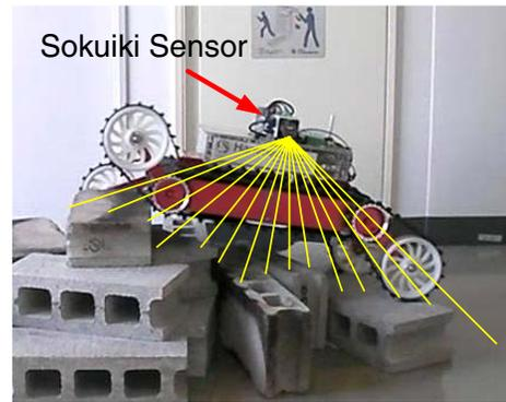
Fig. 6. Terrain sensing using laser range finder
