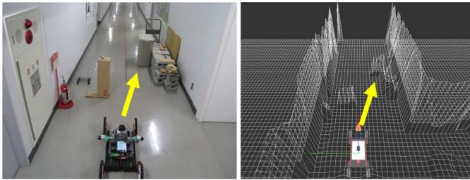
Fig. 5. Teleoperation system based on indication of a waypoint (lower image) and the corresponding real-world scene (upper image)
