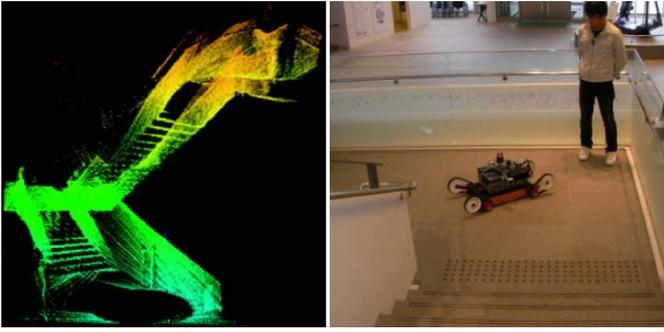
Fig. 10. Image obtained using point cloud data (left) for the stairs (right)
