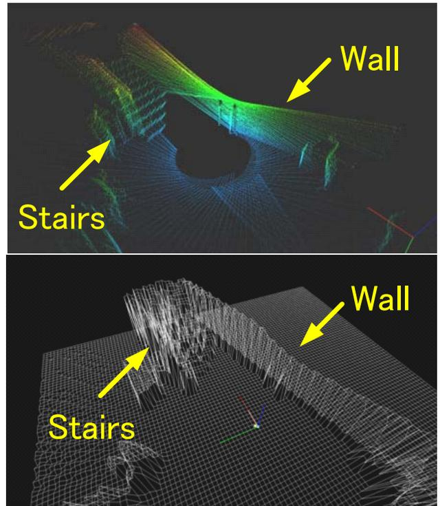
Fig. 4. Environment expression: Point cloud representation (upper image) and DEM (lower image)
