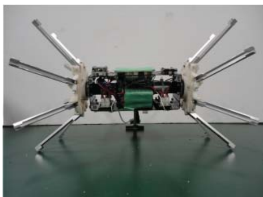
Fig. 2: New model of a mobile robot with expandable wheels
