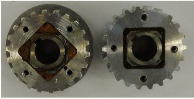
Fig. 8. Impact absorption mechanism. The left side of the photograph shows the original one, which is broken. The absorption material is offset to the corners, and a phase shifting occurs (about 45 degree). The right side of the photograph shows the improved version.
