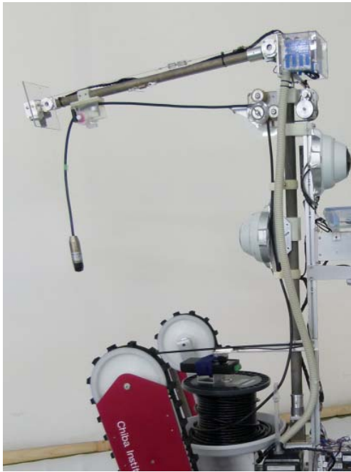
Fig. 6. Photograph of developed 2 DOF manipulator with water gauge.
