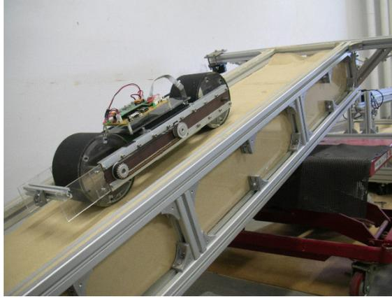
**Figure 7. Two-wheeled rover travels over a slope.**
