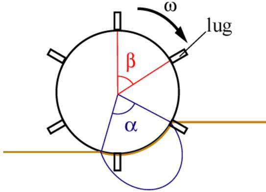
**Figure 2. Angle where lugs develop thrust,  $\alpha$ , and angle between lugs,  $\beta$ .**
