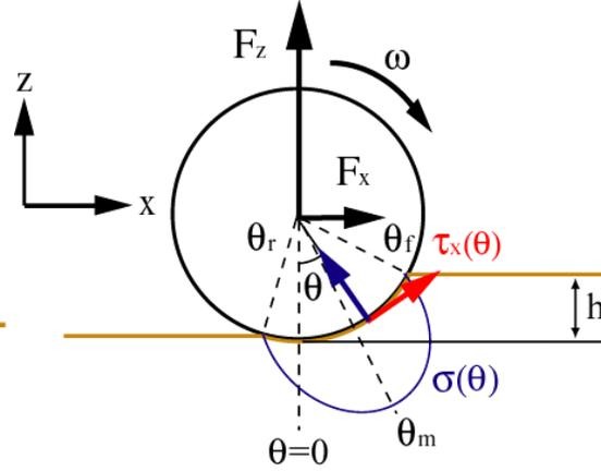
**Figure 3. Normal stress  $\sigma$  and shear stress  $\tau_x$  generated beneath wheel.**
