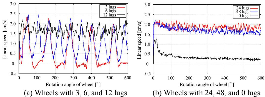
**Figure 9. Rotation angle of wheel versus linear traveling speed (for 15mm-height lug).**
