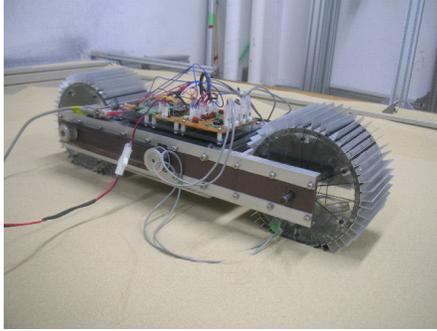
**Figure 5. Two-wheeled rover.**
