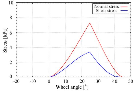
**Figure 4. Normal and shear stress distribution beneath a wheel without lugs, which has a diameter of 150 mm and a width of 100 mm (normal load of the wheel was 2.0 kg).**
