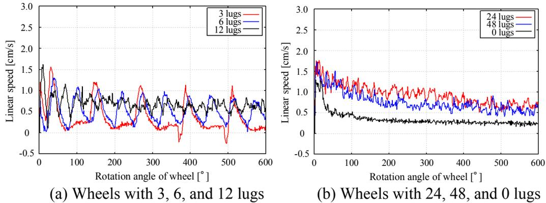
**Figure 8. Rotation angle of wheel versus linear traveling speed (for 5mm-height lug).**
