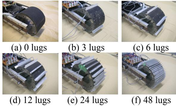
**Figure 6. Wheels equipped with different numbers of lugs.**
