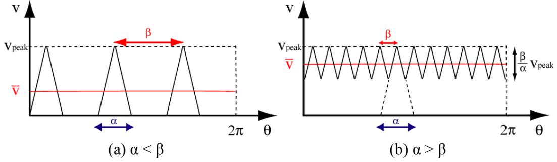
**Figure 1. Linear traveling speed of wheels with lugs;  $\alpha$  and  $\beta$  denote an angle where lugs develop thrust and an angle between lugs, respectively.**
