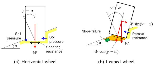
Fig. 13. Gravitational forces based on the wheel contact conditions, and a slope failure resulting due to wheel rotation
