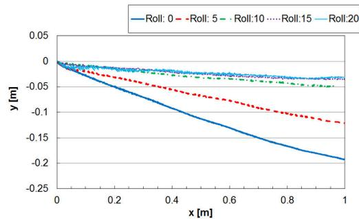
Fig. 11. Experimental traversal paths in slope coordinate (slope angle, 15 [deg]; rovers mass, 23.8 [kg])
