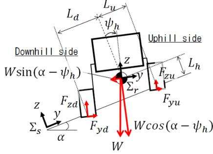
Fig. 2. Mechanical rover model on a side slope
