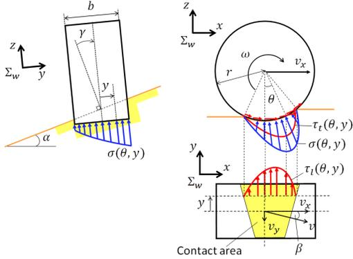
Fig. 4. Normal and shear stresses beneath a wheel
