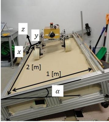
Fig. 10. Test field filled with dry loose sand
