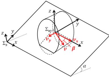
Fig. 3. Wheel coordinate system on a lateral slope
