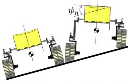
Fig. 9. Rover test bed and its reconfiguration (left: nominal configuration, right: inclined configuration)
