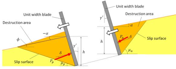
Fig. 7. Passive and active soil resistances on the sidewall
