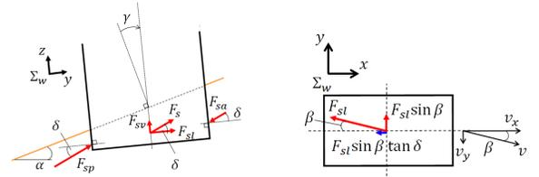
Fig. 8.  $x$ ,  $y$ , and  $z$  components of  $F_s$
