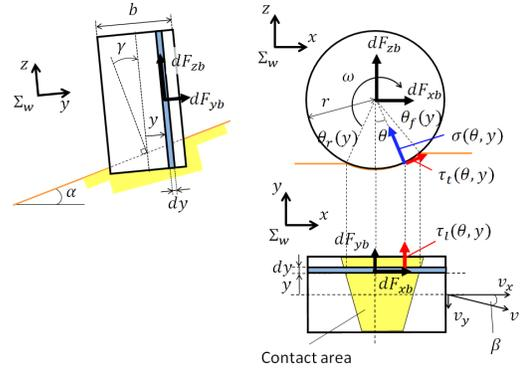
Fig. 5. Forces acting on a sliced wheel element
