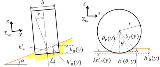
Fig. 6. Sinkage of a tilted wheel on a slope
