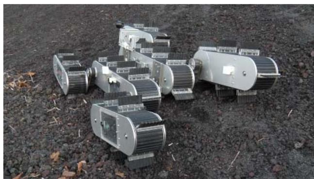
Fig. 2. Novel design of tracked vehicle ELF, which consists of two main tracks and four subtracks. It is equipped with a total of eleven mounted actuators that give it a high degree of traversability on weak and uneven terrains.
