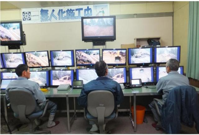
Fig. 5. Recent teleoperation room for unmanned construction
