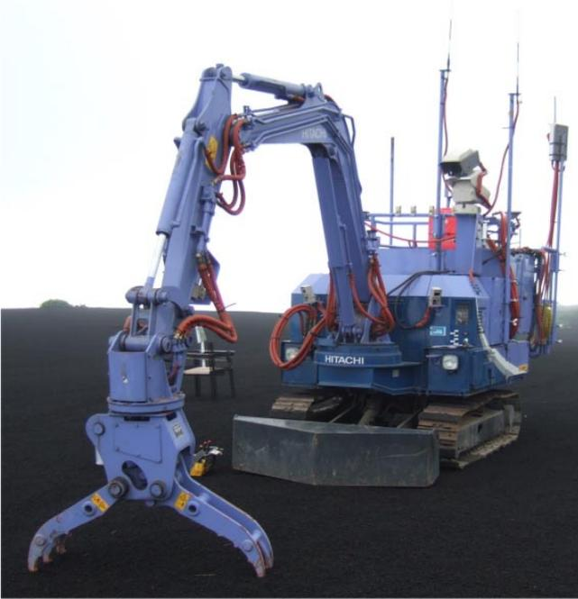
**Fig. 3.** Volcano observation robot “MOVE”
