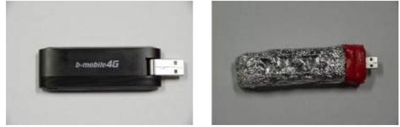
Fig. 7: Before (left) and after (right) covering the 3G device with aluminium
