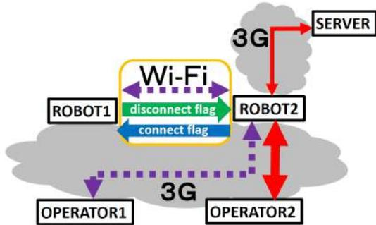
Fig. 3: Teleoperation of robots via a 3G/Wi-Fi combination
