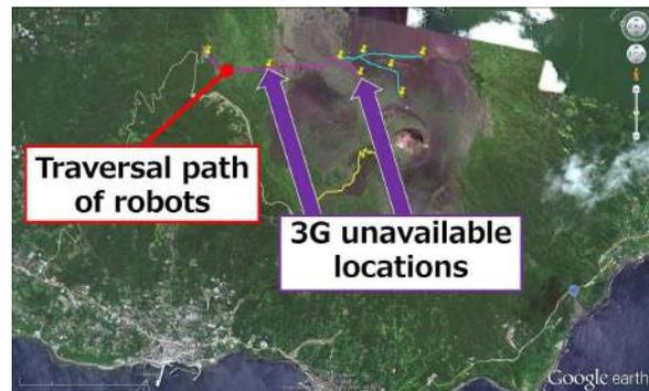
Fig. 1: Traversal path of robots and the locations at which the robots failed to communicate with the operator via the 3G network on Mt. Mihara
