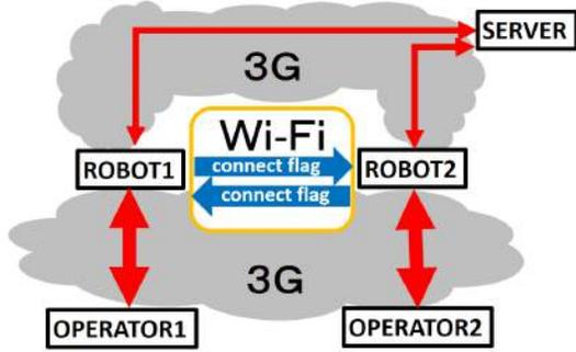
Fig. 2: Teleoperation of two robots via 3G network
