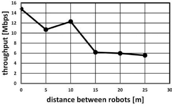
Fig. 6: Communication throughput between robots
