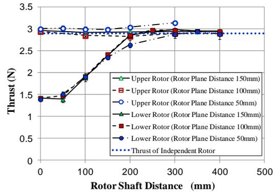
Figure 10. Thrust of overlapping rotors.
