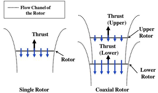
Figure 3. Flow model of an isolated rotor and a coaxial rotor[2].
