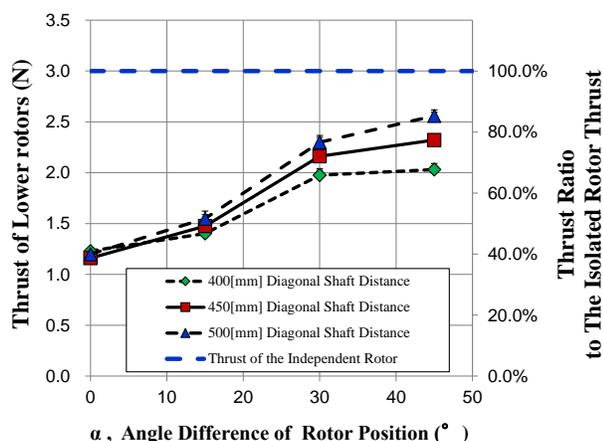
Figure 17. Thrust of a lower rotor in different configuration at 6000rpm.
