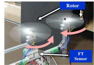
Figure 7. Biaxial rotor measurement.
