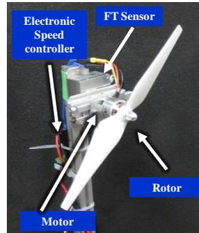
Figure 6. A rotor and a force torque sensor.
