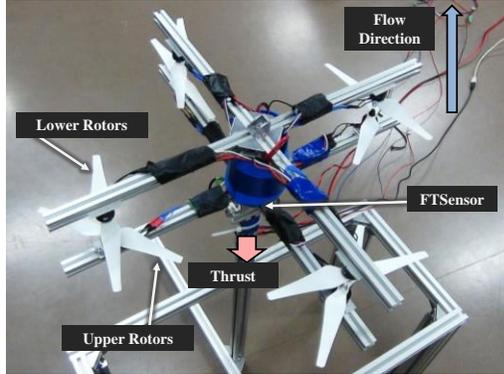
Figure 14. Measurement of octorotor UAV model thrust changing an angle of rotor planes.
