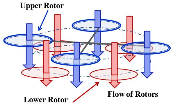
Figure 12. Concept of octorotor UAV avoiding wake interactions.
