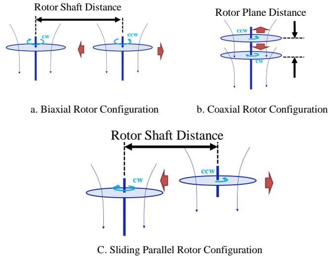
Figure 4. Rotor relative positions in the experiment.
