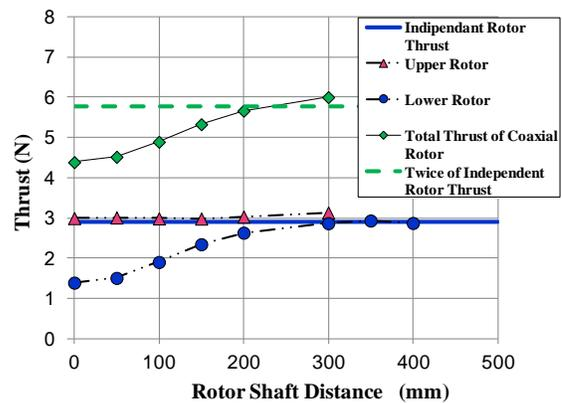
Figure 11. Thrust of overlapping rotors.
