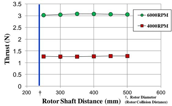
Figure 8. Thrust of biaxial rotors.
