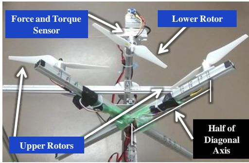
Figure 13. Measurement of thrust on two upper rotors and a lower rotor.
