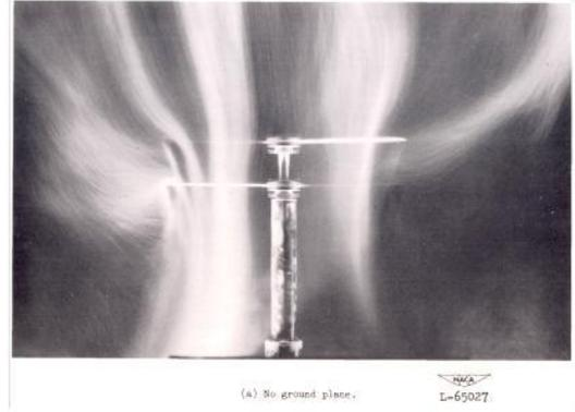
Figure 2. Visualized flow of coaxial rotor[1].
