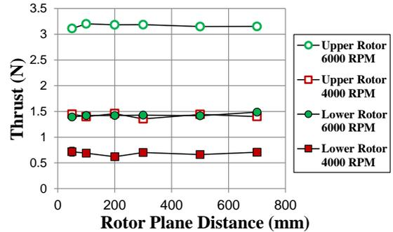
Figure 9. Thrust of coaxial rotors.
