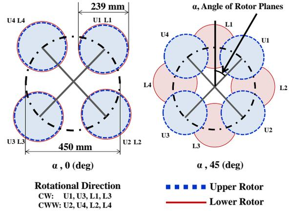
Figure 16. Top view of rotor arrangement for two angles at 450mm diagonal axis distance.
